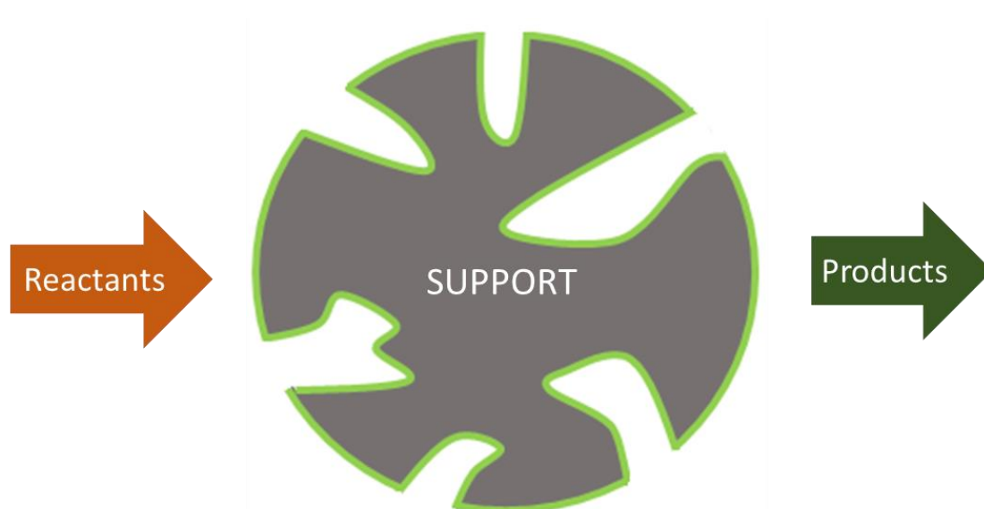
Figure 1 - Schematic representation of supported IL; the green line represents the IL phase containing a homogeneous catalyst.
